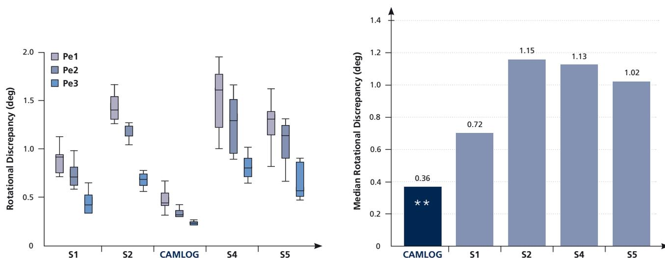
**Rotational Discrepancy.** Five implant systems were tested: S1, S2, S4, S5, and CAMLOG. Pe1, 2, and 3 represent results from three independent test persons. Figure adapted from Fig. 4 of Semper et al., 2010.
